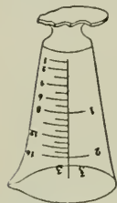
Graduate (chipped and broken base)
