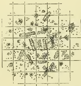
Microscopic Appearance of Common Calcined Magnesia.
