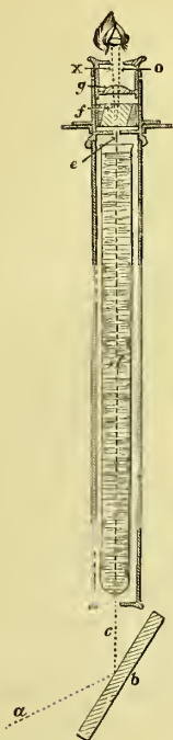
Plan of the Apparatus for showing the circular polarization of liquids.
